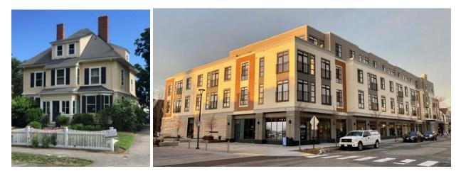
*Left: Example of a pitched roof half-story Right: Example of a stepped back flat roof*
