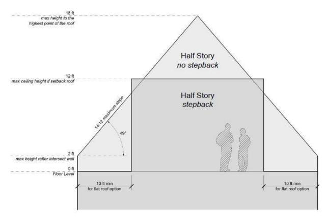
Above: Diagram to define half-story condition for a flat roof or pitched roof
