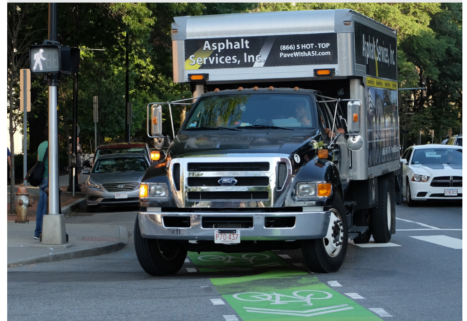
Design vehicle negotiating an intersection corner
