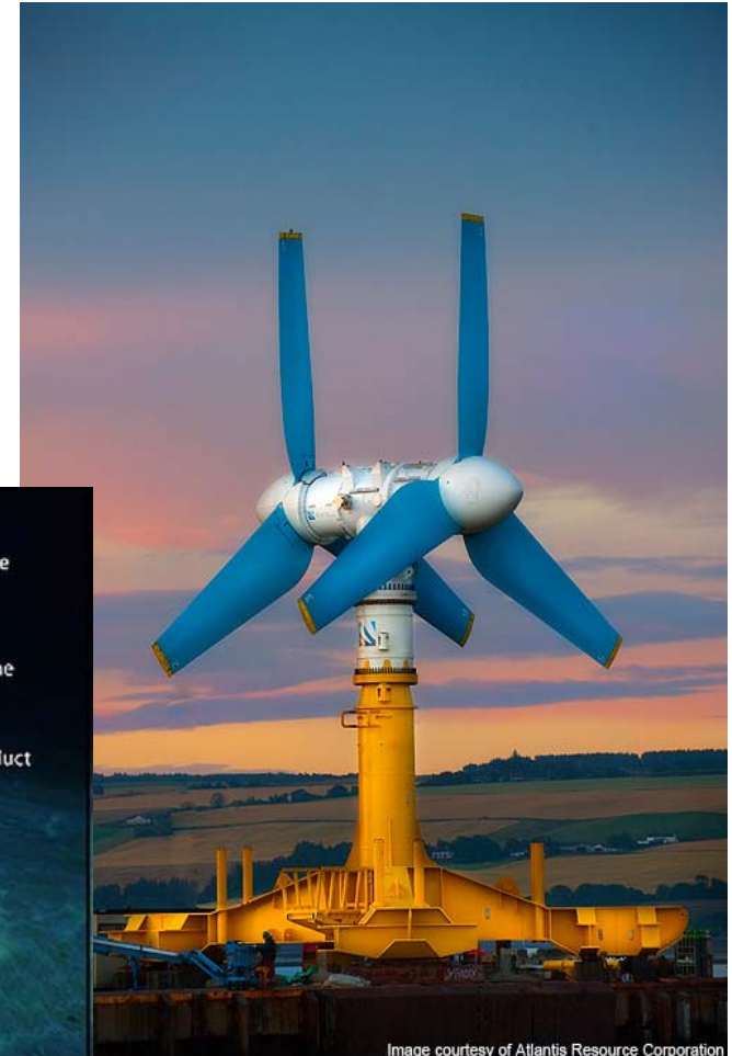
AK-1000 Tidal Turbine 1 and 2 MW, United Kingdom
