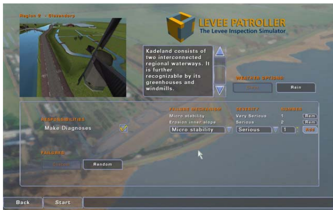
Figure 6. Screenshot of the scenario generator. The region, weather, types of responsibilities and failures can be chosen.
