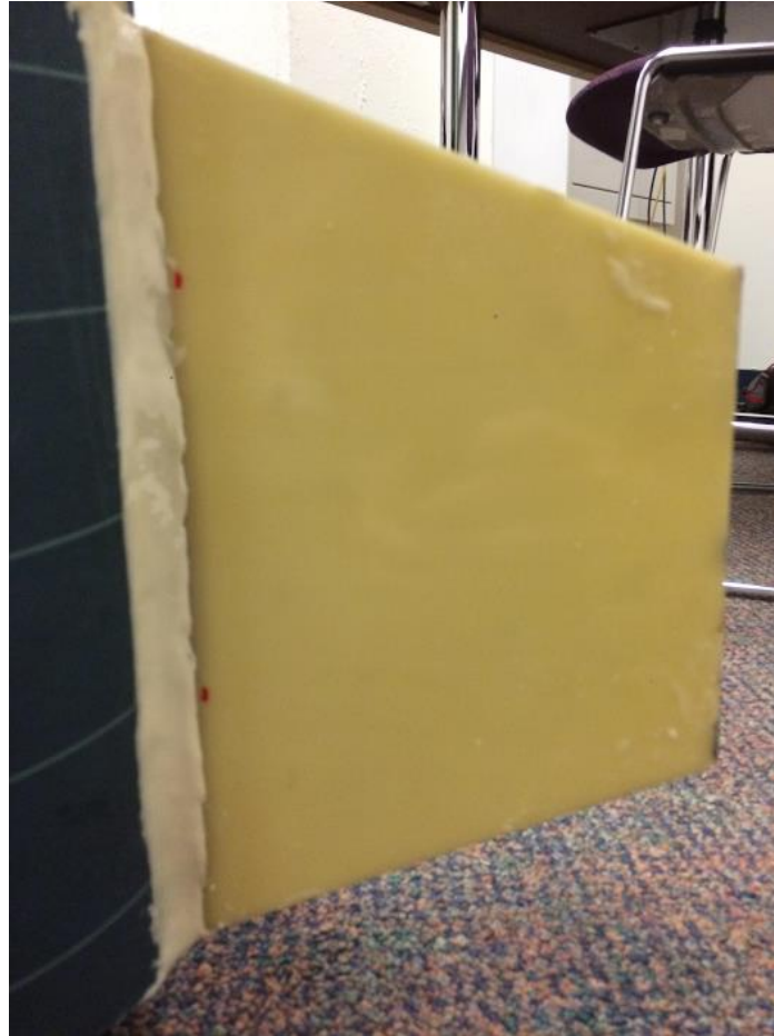
Figure 4 G10 Fiberglass Fins
