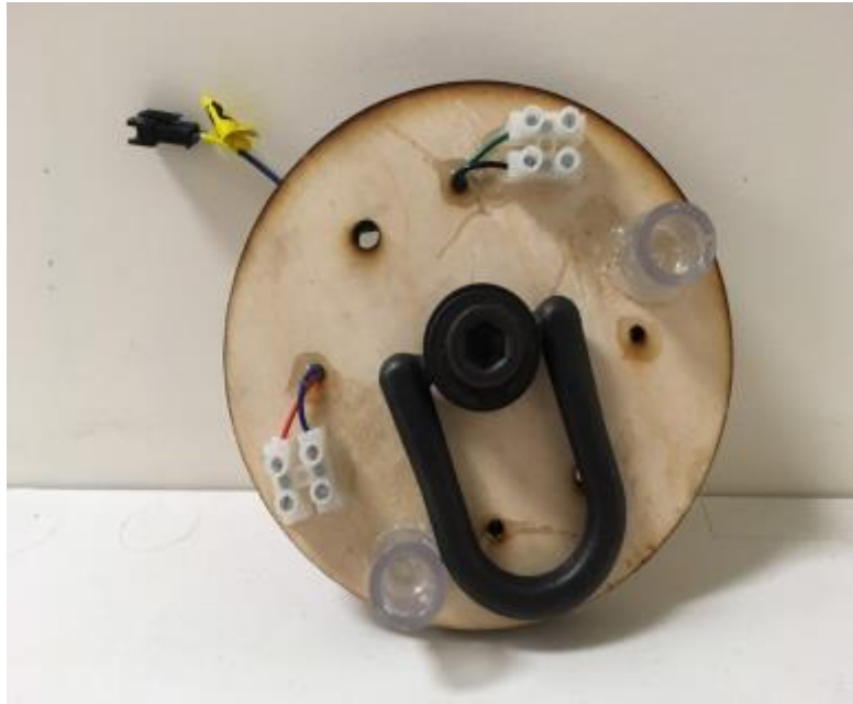
Figure 3 Electronics Bay Main Parachute Bulkhead
