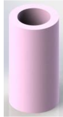
Figure 54 Horizontal Dampening Foam (Radial)
